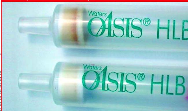
Figure 3: Left-side column (SPE Step 1): The column on the left shows the retained matrix resulting from the initial sample pass-through. This column is discarded and the passed-through sample is then derivatized. Right-side column (SPE Step 2): The column on the right shows the sample clean-up after the final analyte elution.
