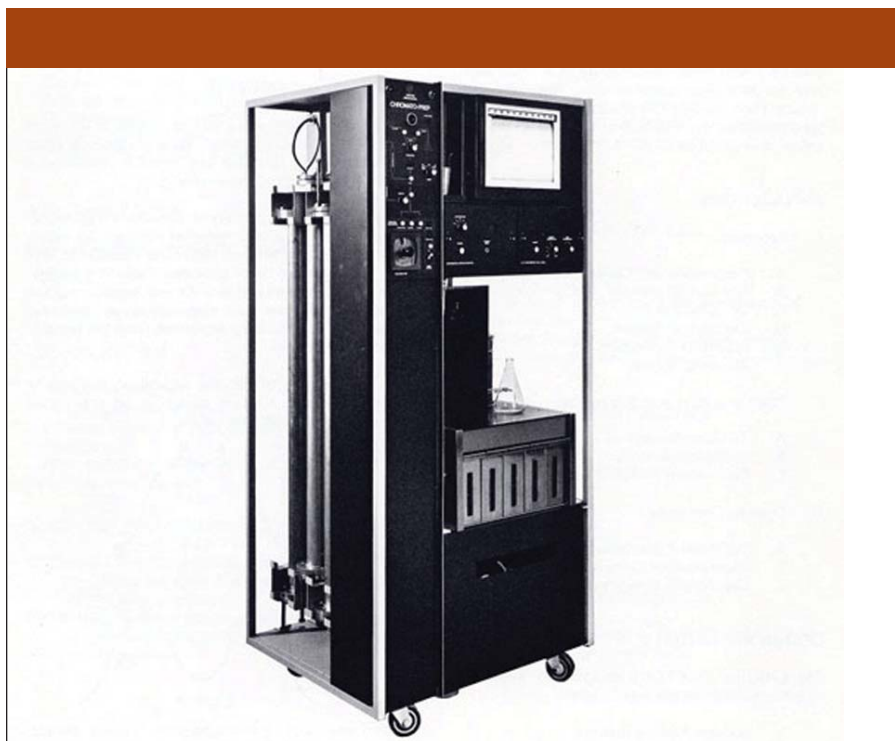
Figure 6: The Chromato-Prep GPC-LC instrument for preparative-scale work, introduced in 1968. The column compartment is open, showing four columns installed. Below the space in the middle of the right side of the module is a fraction collector, while the two-pen potentiometric recorder is installed in the right top.
