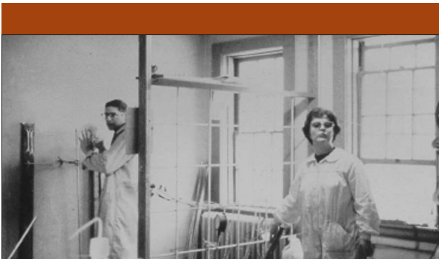
Figure 1: The laboratory of Waters Associates in 1963, established in the female detention area of the former Framingham police station. Right, in forefront, technician Nicky Anastis is stirring a batch of the PS-DVB mixture used to synthesize the Styragel column packing. The reaction vessel was fabricated by Jim Waters from a standard, 55-gallon metal drum.
