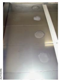
Figure 1: Representative residues on stainless steel.
