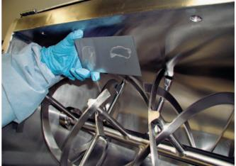
Figure 2: Equipment inspection using spotted plates.
