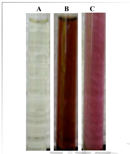
Figure 1. Biosynthesis of gold nanoparticles (GNPs): A) auric chloride (HAuCl 4 ) solution, B) extract, C) synthesized GNP in ruby red color solution.
