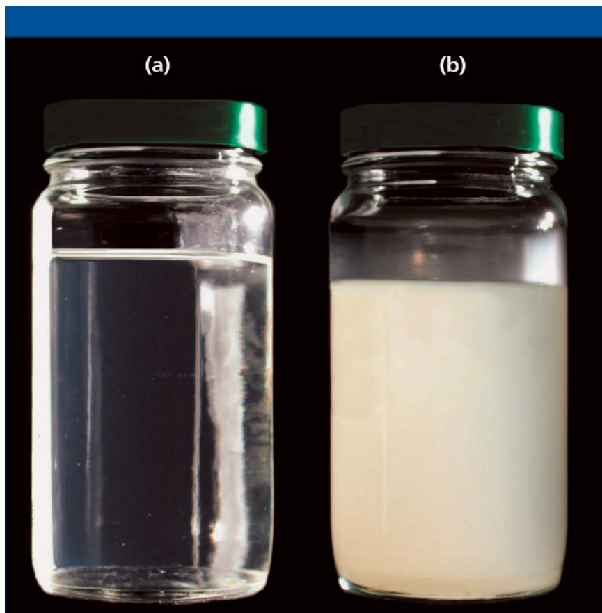
Figure 1: (a) Clear (least hazy) transparent monomer solution; (b) haziest monomer solution.
