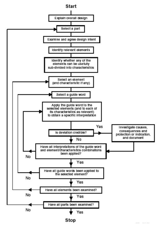
The following figure graphically illustrates the HAZOP Examination Phase process flow.<sup>1</sup>
