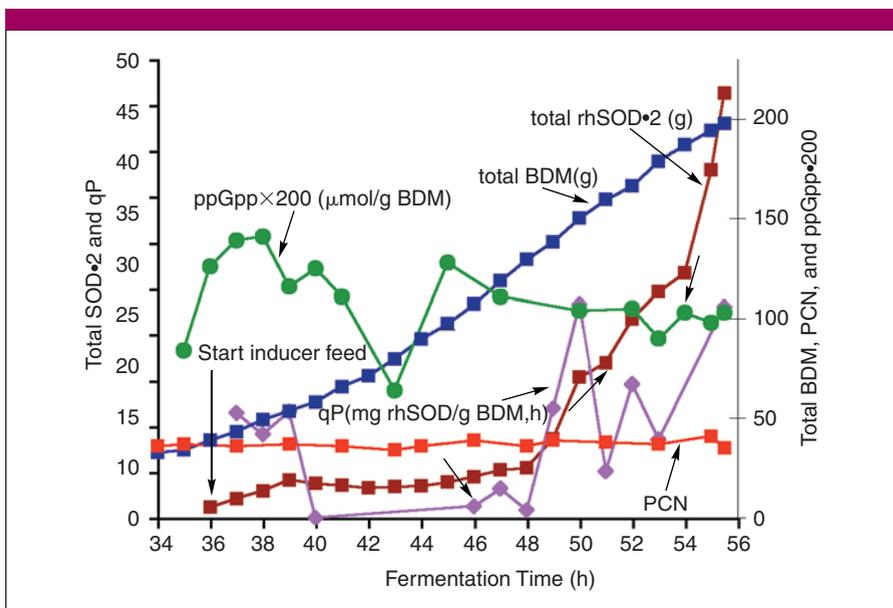
**Figure 3.** Fed-batch process for the production of recombinant human superoxide dismutase using modified *E. coli* (HMS174(DE3)pET11ahSODclone3); shows stabilized plasmid replication; exponential substrate feed with a growth rate of  $0.1 \text{ h}^{-1}$ ; inducer feed ( $\mu\text{mol IPTG/g BDM}$ ) was increased in three steps to assess stability of the plasmid copy number: 0.6–1.17 at 35–43 h, 1.17–3.26 at 43–48 h, and 3.26–19.6 at 48–55 h.
