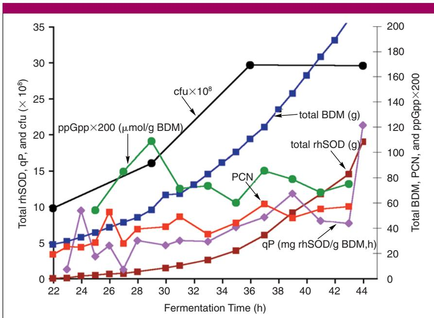
**Figure 5.** Fed-batch process for the production of recombinant human superoxide dismutase using modified *E. coli* (HMS174(DE3)pET11ahSOD) with a continuous feed of inducer (lactose) to control transcription rate
