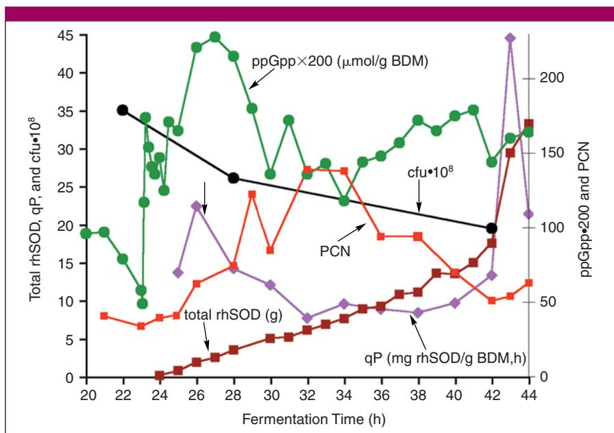
**Figure 4.** Fed-batch process for the production of recombinant human superoxide dismutase using modified *E. coli* (HMS174(DE3)pET11ahSOD) with a continuous feed of inducer (IPTG) to control transcription rate
