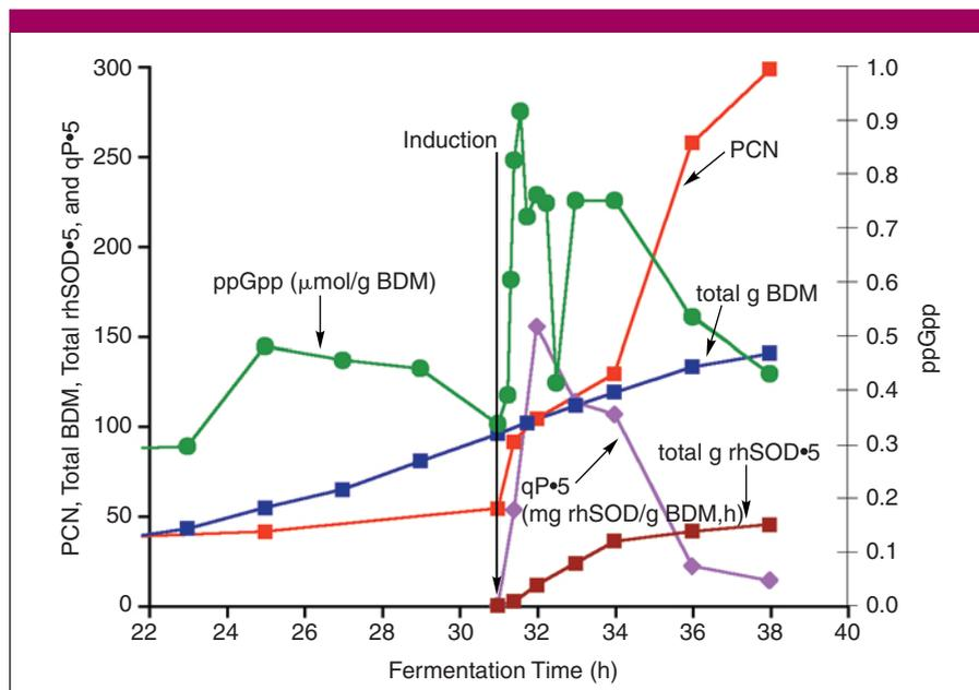
**Figure 1.** Standard fed-batch process for the production of recombinant human superoxide dismutase using *E. coli* (HMS174(DE3)pET11ahSOD) with a growth rate of  $\mu = 0.1 \text{ h}^{-1}$  maintained by exponential feed
