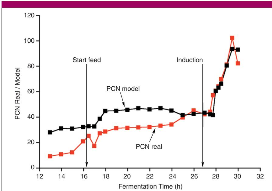
**Figure 2.** Modeling of plasmid copy number (PCN) from online data uses neural network simulations. Fed-batch fermentation of *E. coli* (HMS174(DE3)pET11ahSOD) has an exponential feed of  $\mu = 0.2 \text{ h}^{-2}$ .
