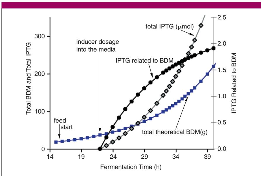
**Figure 6.** Model-based determination of appropriate amounts of inducer (IPTG) in ratio with the biomass in a fed-batch process for maximum exploitation of the host cell metabolism
