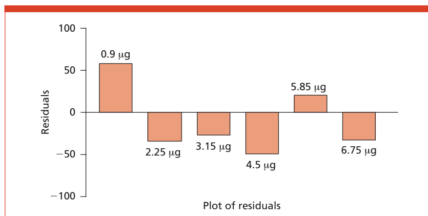
Figure 4: Test for linearity of calibration graph by plotting the residuals in the working range.
