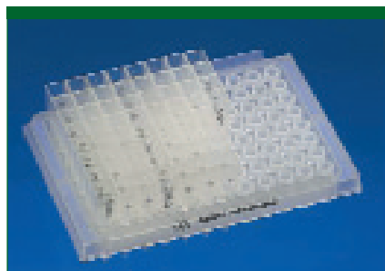
Figure 4: Photograph of a flexible 96-well SPE plate with removable cartridges and plug strips. (Courtesy of Agilent Technologies.)
