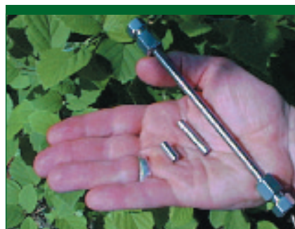
Figure 5: Photograph of a regular-length HPLC column (25 cm) and short, fast 1 and 3 cm HPLC columns. (Courtesy of Agilent Technologies.)
