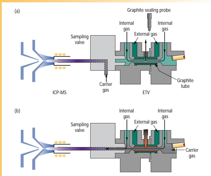
**Figure 1.** A graphite furnace ETV sampling device for ICP-MS, showing the two distinct steps of (a) sample pretreatment and (b) vaporization into the plasma. (Courtesy of PerkinElmer Instruments, Shelton, CT.)
