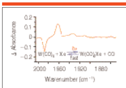
Figure 6. Spectral slice at 10 ns of photo-induced chemical reaction taken from a four-scan, 2-h step-scan TRS data collection.
