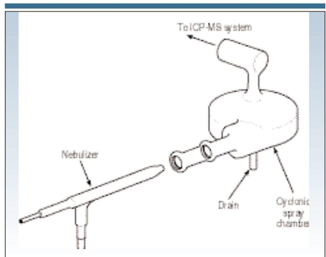
Figure 9. Schematic of a cyclonic spray chamber (shown with concentric nebulizer).
