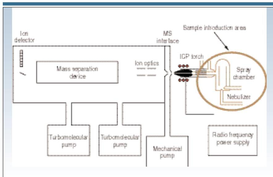
Figure 1. ICP-MS system diagram showing the location of the sample introduction area.
