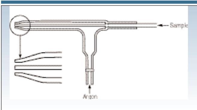
Figure 5. Diagram of a typical concentric nebulizer.
