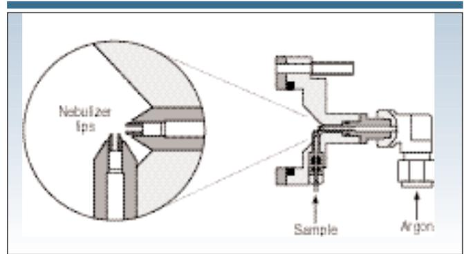
Figure 6. Schematic of a crossflow nebulizer.
