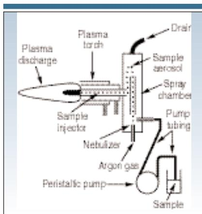
**Figure 2.** Diagram of the ICP-MS sample introduction area.
