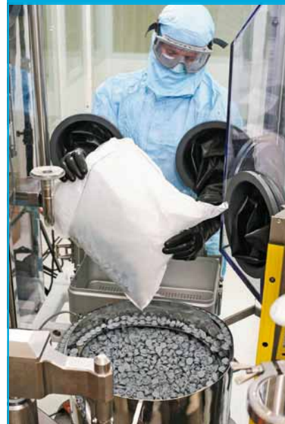
Figure 2: Glove ports are used for a filling operation.
