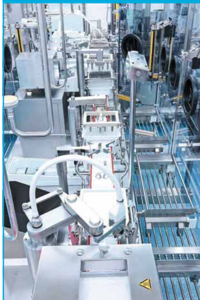
Figure 1: A commercial restricted barrier access system (RABS).
