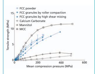
**Figure 4:** Tensile strength vs. mean compression force for tablets formulated with paracetamol and one of the following: functionalized calcium carbonate (FCC) powder or microcrystalline cellulose (MCC). The tensile strength of FCC tablets was comparable to that of tablets formulated with MCC.
