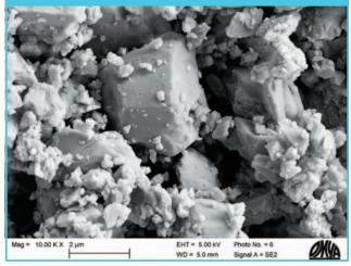
**Figure 2:** Micrograph of functionalized calcium carbonate.
