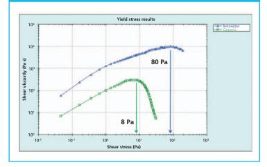
Figure 5: Viscosity vs shear rate for acyclovir creams.
