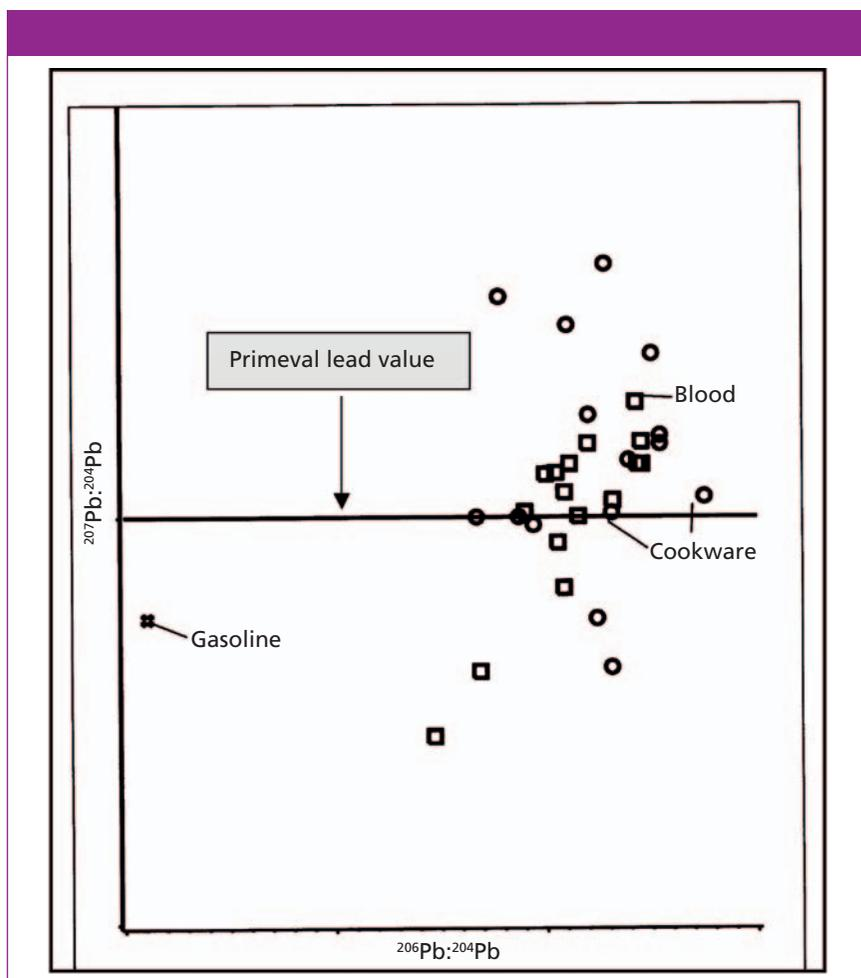
**Figure 6:** A plot of the ratio of  $^{206}\text{Pb}:^{204}\text{Pb}$ , against the ratio of  $^{207}\text{Pb}:^{204}\text{Pb}$  for blood ( $\square$ ), cookware ( $\circ$ ), and gasoline ( $\times$ ) samples, showing the theoretical (primeval) lead line. Adapted with permission from reference 21.
