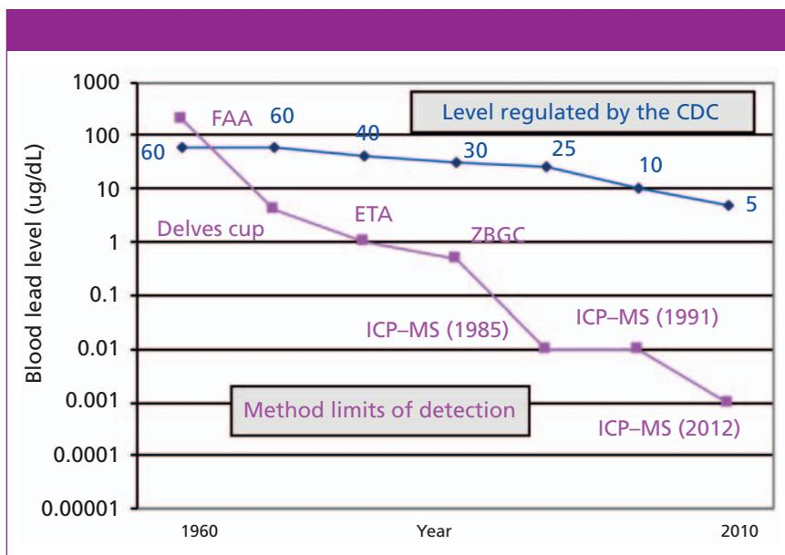
**Figure 3:** The improvement in real-world method detection capability (in  $\mu\text{g/dL}$ ) offered by atomic spectroscopy techniques for blood-lead determinations compared to the trend in blood-lead levels regulated by the Centers for Disease Control and Prevention (CDC).
