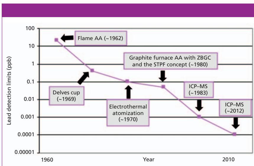
**Figure 2:** Comparison of detection capability (ppb) of atomic spectroscopy techniques used to monitor blood lead and the approximate year they were developed or improved.
