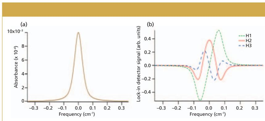
**Figure 2:** At left, an absorption line with 1% absorbance modeled with a Voigt profile; at right, the harmonic signals that would be measured with wavelength modulation (as described in the text) at 1, 2, and 3 times the modulation frequency.
