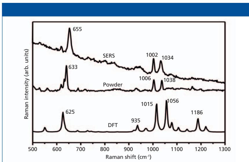
Figure 4: Raman analysis of phenobarbital: theory-calculated, powder, and SERS spectra of an aqueous solution (0.1 mg/mL).
