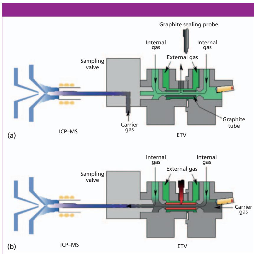
**Figure 5:** Schematic of ICP-MS coupled with an the electrothermal vaporization sampling accessory (ETV-ICP-MS), showing the two distinct stages: (a) pre-vaporization to drive off the matrix components and (b) vaporization to sweep the analyte vapor into the ICP-MS instrument for analysis. Adapted with permission from reference 22.
