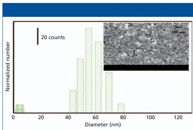
**Figure 2:** Size distribution of silver nanoparticles (inset: SEM picture of silver nanoparticles).
