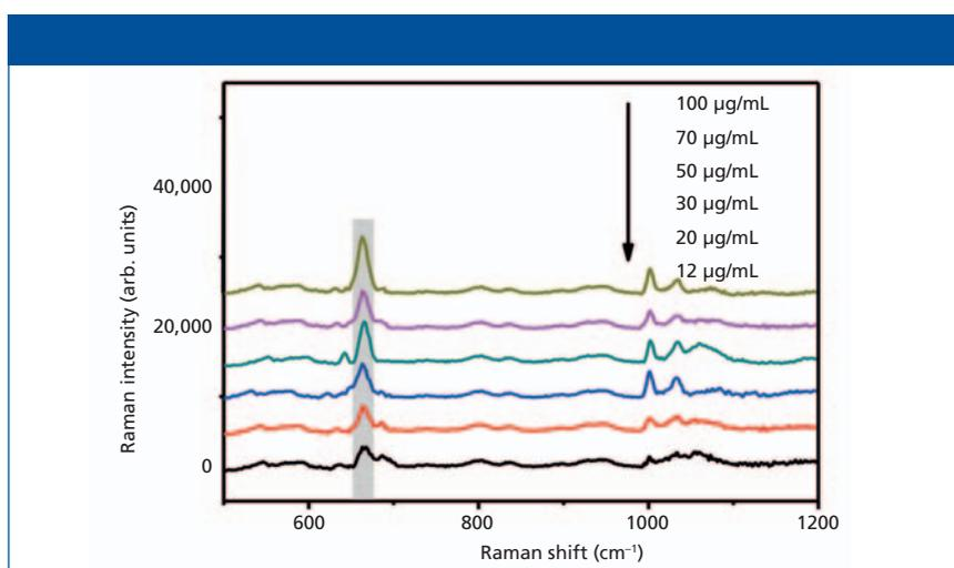
**Figure 6:** SERS spectra of different concentrations of aqueous phenobarbital.
