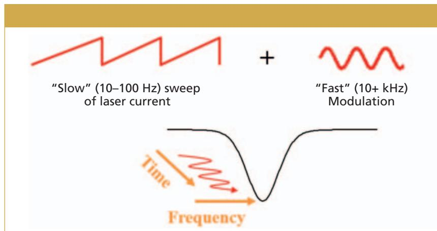
**Figure 1:** Wavelength modulation includes a slow sweep (left) and a faster modulation (right) of the drive current, sweeping across an absorption feature of interest (bottom).
