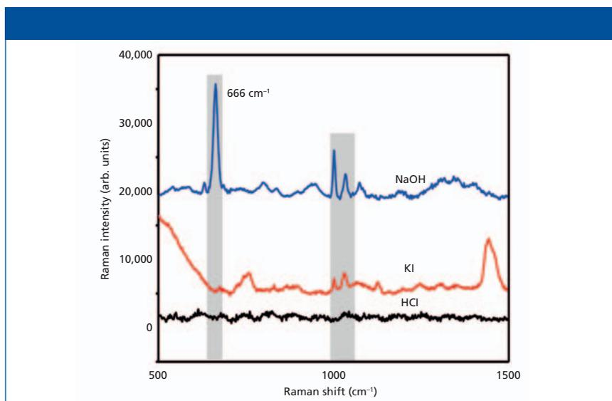
**Figure 5:** SERS spectra of phenobarbital sodium using different aggregating agents.
