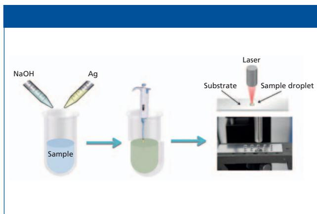
**Figure 1:** Schematic diagram of the method proposed for the phenobarbital detection process.
