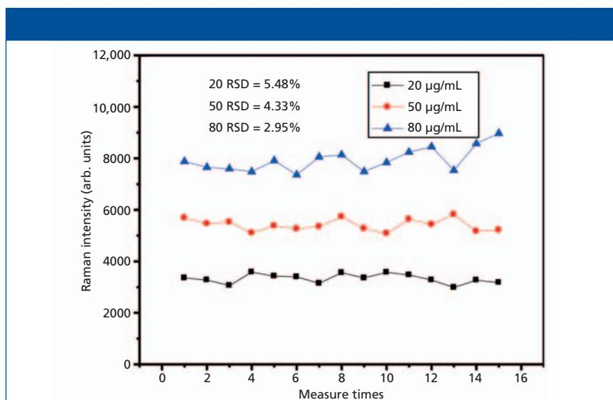
**Figure 7:** Reproducibility of NaOH-induced silver aggregates in solution.
