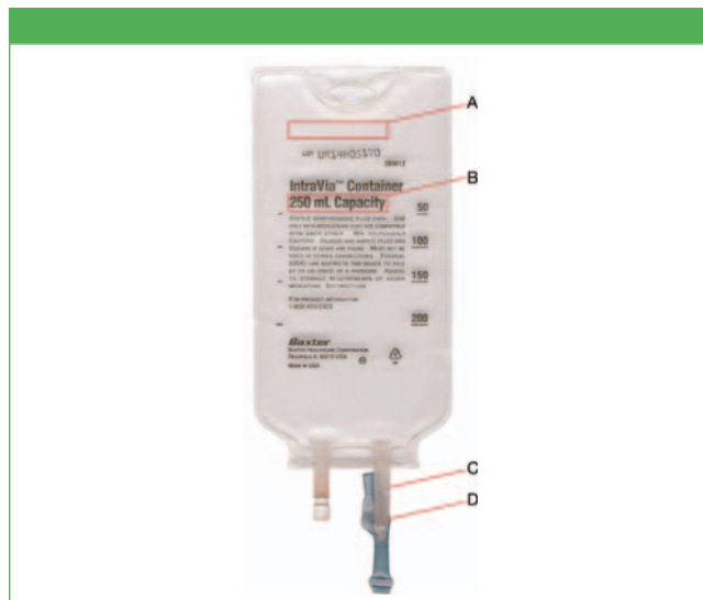
Figure 1: IV bag sampling spots: IV bag sample (A), IV bag sample with imprint (B), tubing (C), and valve (D).
