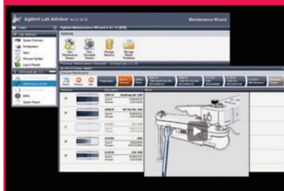
Figure 5: A screen shot of Agilent's Maintenance Wizard showing details of the various modules in the HPLC system and a link to a video illustrating a maintenance procedure to the user.
