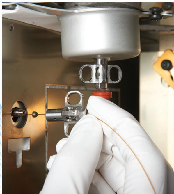
Self Tightening Column Nut for MS transfer line
