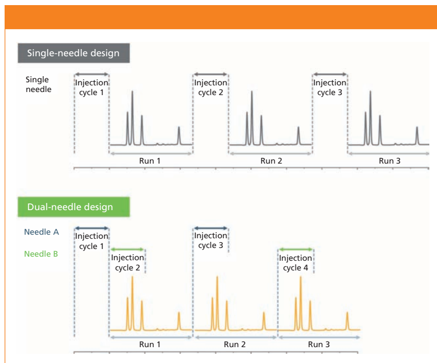
Figure 1: Two comparative signal traces of the reduced cycle time of the Agilent 1290 Infinity II system using the new Multisampler autosampler with a dual-needle design that eliminates time lags between injections.
