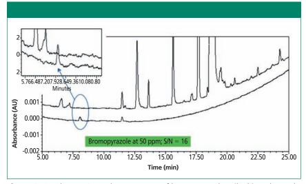
**Figure 3:** Overlay HPLC–UV chromatogram of bromopyrazole spiked in a drug substance. Column: 150 mm  $\times$  4.6 mm, 3.5- $\mu$ m Zorbax Eclipse XDB-C18 Rapid Resolution.
