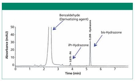
**Figure 5:** A representative chromatogram for analysis of hydrazine and isopropyl hydrazine. Column:  $150 \text{ mm} \times 4.6 \text{ mm}$ ,  $3.5\text{-}\mu\text{m}$  Waters Xbridge C18; mobile-phase A: water; mobile-phase B: acetonitrile; temperature: 50 °C; injection volume:  $5 \mu\text{L}$ ; flow rate: 1 mL/min.
