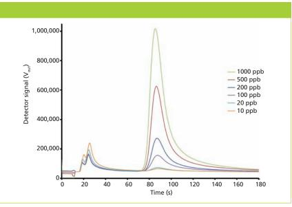
Figure 3: An overlay of chromatograms ranging from 10 to 1000 ppb (v/v) of ethylene in air.
