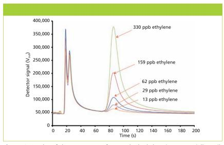
**Figure 6:** Overlay of chromatograms of entrenched ethylene in commercially available industrial solvents.
