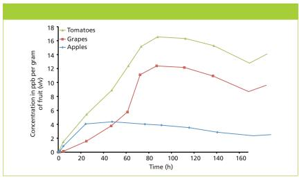
**Figure 4:** A plot of the amount of ethylene generated by various matrices over the course of 168 h (seven days).
