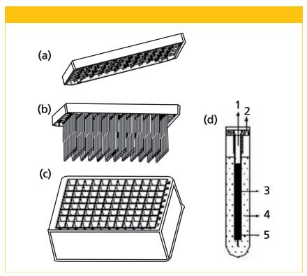
**Figure 1:** Hollow-fiber microextraction in a 96-well format: (a) the plastic base, (b) the attachment of hollow fiber to the plastic base, (c) the 96-well plate, and (d) an expanded view of the hollow-fiber device. 1 = hollow-fiber attachment tip, 2 = donor phase collection tip, 3 = acceptor phase, 4 = donor phase, 5 = hollow fiber. Adapted with permission from reference 2.
