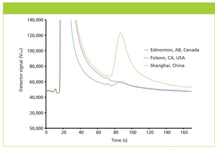
**Figure 5:** Overlay of chromatograms of ethylene in air from three different locations.
