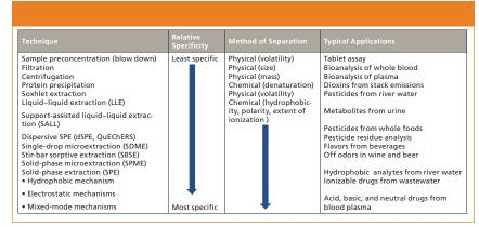
**Figure 1:** Description of the various commonly used sample preparation techniques. Note that the list of typical applications is for illustrative purposes only and is not meant to be exhaustive.
