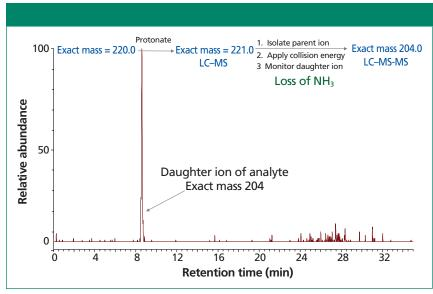
**Figure 4:** Representative chromatogram of hydroxylamine impurity MRM at 1 ppm level.
