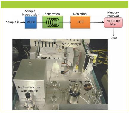
Figure 1: A block diagram of the analytical system.
