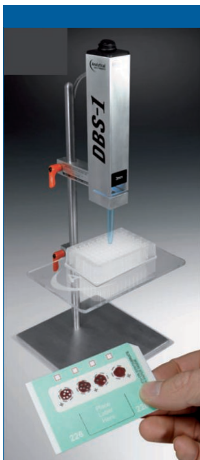
Figure 4: Dried blood spot pneumatic card punch. (Courtesy of Analytical Sales and Services.)
