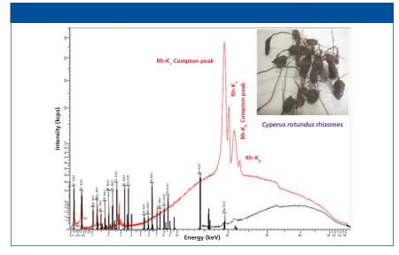
**Figure 5:** Typical WD-XRF spectrum of *Cyperus rotundus* (snapshot shown in inset) in different energy regions indicating the presence of macro- and micronutrient minerals. Details about spectral information can be found in reference 4.
