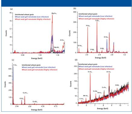
**Figure 3:** Typical WD-XRF spectra of uninfected and infected wheat grains in energy ranges (a) 0.5–1.5 KeV indicating the presence of Mg and Al; (b) 1.7–3.3 KeV indicating the presence of Si, P, S, and Cl; (c) 3.3–5 KeV indicating the presence of K and Ca; and (d) 5–11 KeV indicating the presence of Cr, Mn, Fe, Ni, Cu, and Zn. Adapted with permission from reference 3.
