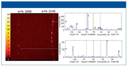
**Figure 2:** Example of a 2D X-ray detector image of coarse-grained steel. On the right-hand side the result of the automatic spot detection for the {110} and {200} reflexes is given.
