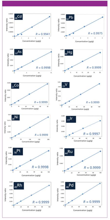
Figure 1: The calibration curves for Cd, Pb, As, Hg, V, Co, Ni, Ir, Pt, Ru, Rh, and Pd.
