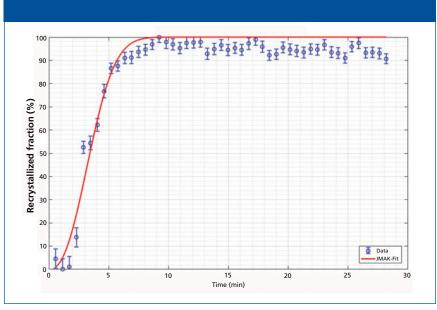
**Figure 1:** Recrystallized fraction of a dual-phase steel annealed at 700 °C. The fractions are derived from the width of the {110} Bragg reflex measured with in situ XRD.
