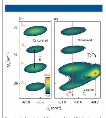
**Figure 1:** (a) Calculated and (b) measured 1213 RSMs for 20 periods GaN–AlN SLs with the following superstructure parameters:  $T_{\rm SL}=9.46$  nm;  $t_{\rm GaN}/t_{\rm AlN}=4.38/5.08$  nm;  $\varepsilon_{\rm x}$  (GaN–AlN)= -3.05  $\times$  10<sup>-3</sup>/1.58  $\times$  10<sup>-3</sup>;  $N_{\rm TD}=3.32 \times 10^8$  cm<sup>-2</sup>. The intensity is plotted in logarithmic scale.
