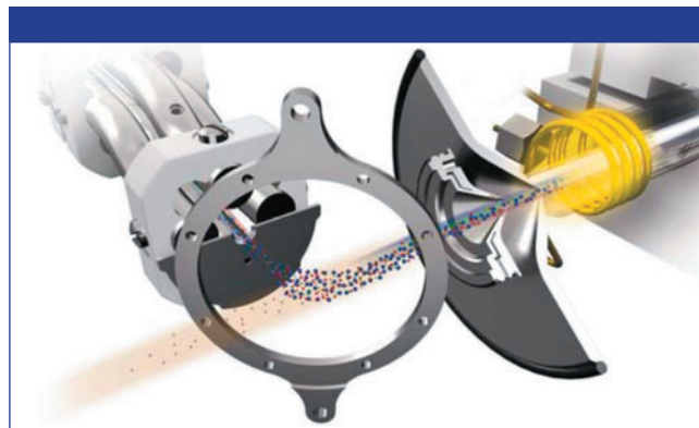
Figure 2: Schematic view of Bruker's ion mirror and off-axis quadrupole fringe rods.
