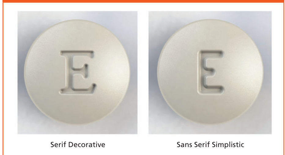
Figure 1. Decorative or serif fonts are more prone to picking problems than simple, sans serif fonts.
