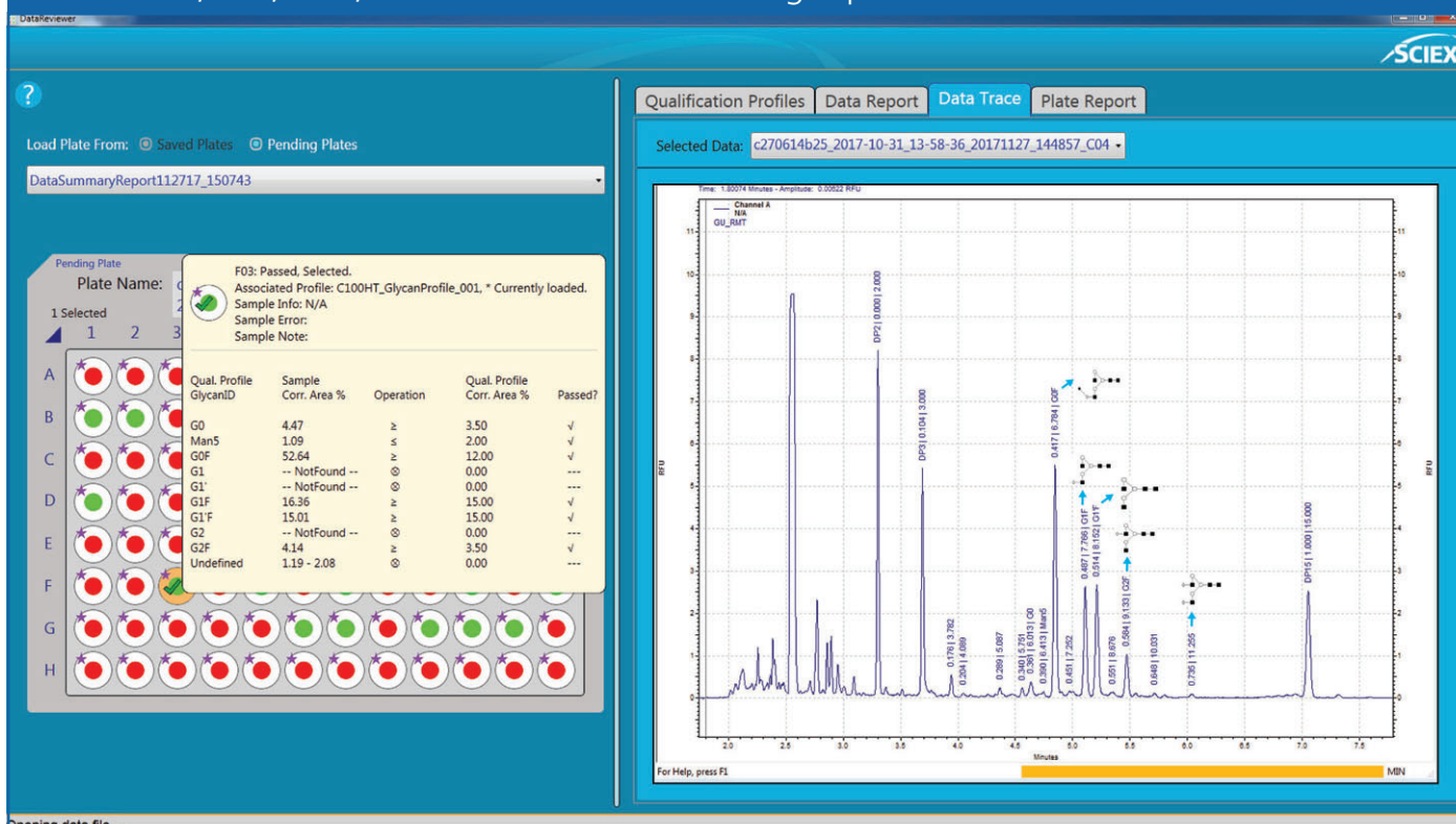
Figure 3: Qualification profile and dynamic pass/fail display of the wells on a 96-well plate. In the left panel of this figure, a plate map in the software illustrates that all 96 samples were selected for data analysis, as indicated by the green check marks. Glycans released from MAK33 were analyzed for corrected peak area percentage between each sample well for G0, G0F, G1F, G1'F, and G2F species. The RSD% for 96 samples is below 9% for G0, and around 6% for G0F, G1F, G1'F, and G2F as shown in the right panel.
