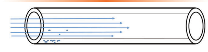
FIGURE 2: Simplified picture of analyte partitioning in a capillary GC column. Analyte molecules are represented by dots. There are nine dots in the stationary phase and three in the mobile phase, giving k = 3 . Reprinted from Reference 2 with permission of the author.
