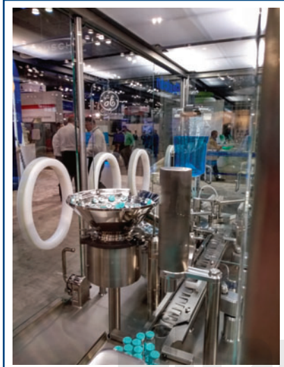
Figure 1: The Flexicon FPC60 fill/finish machine from Watson-Marlow Fluid Technology Group uses a peristaltic pump and custom, precision tubing.
