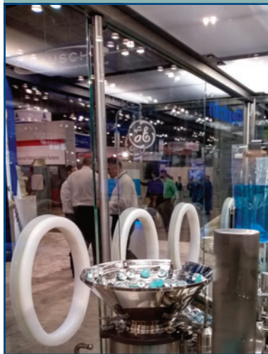
Figure 1: Flexicon FPC60 fill/finish machine from Watson-Marlow Fluid Technology Group uses a peristaltic pump and custom, precision tubing.
