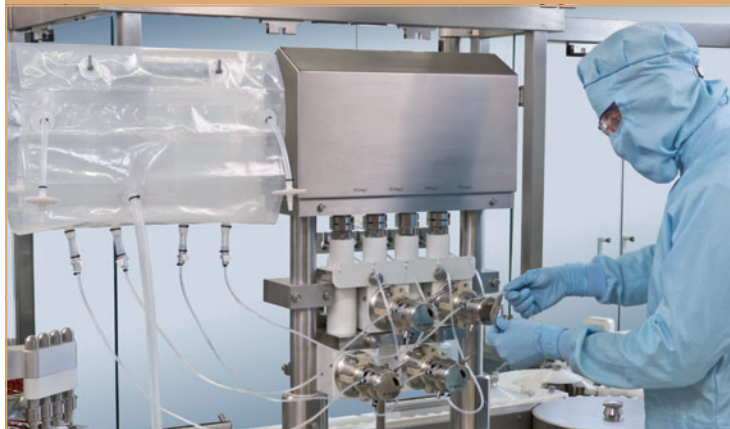
Figure 3: Single-use liquid filling equipment, such as the PreVAS single-use system with peristaltic pump (Bosch Packaging Technology) can be used in either traditional vessels or fully disposable fluid handling technologies.
