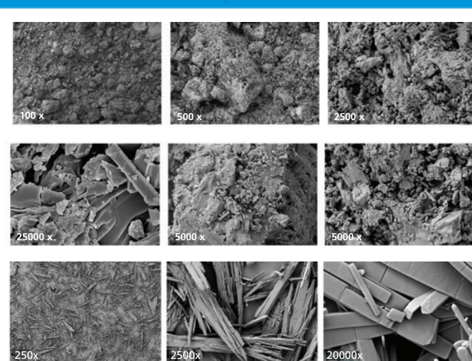
Figure 5: SEM images of Form 1 before (top 6 images) and after (bottom 3 images) morphology development.
