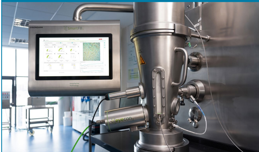
Figure 1. Fluid-bed granulator (Glatt GPCG2) equipped with a particle analyzer (Eyecon2, Innopharma Technology) and near infrared spectrophotometer (Multieye2, Innopharma Technology) with a system user interface (SmartX, Innopharma Technology).
