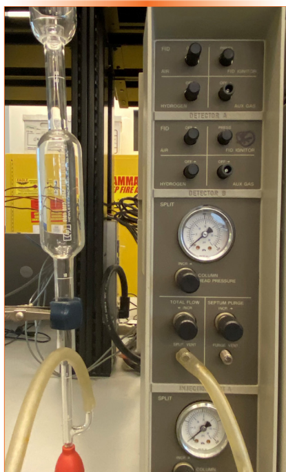
FIGURE 2: Soap film flowmeter connected to the split vent of a classical pneumatic gas chromatograph.
